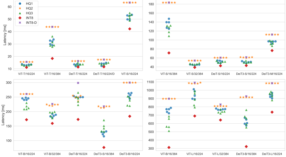
Figure 4.3: Average model inference latency on the A15 Bionic CPU: each point represents a single quantization configuration of the selected HQ algorithm. We compared the latency of the proposed methods with INT8 and INT8-D. The measurements were averaged over 1000 samples.
