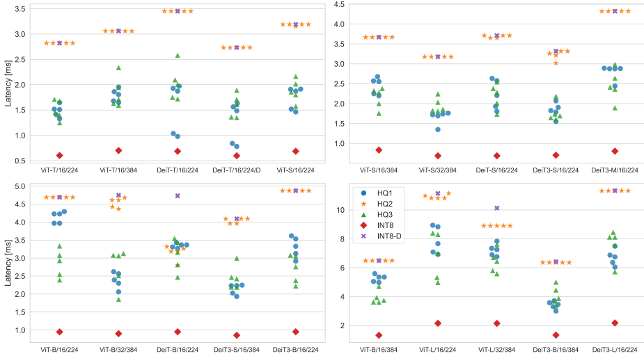
Figure 4.4: Average inference latency of models on the A100 GPU-equipped workstation: each point represents a single quantization configuration of the selected HQ algorithm. We compared the latency of the proposed methods with INT8 and INT8-D. The measurements were averaged over 1000 samples.
