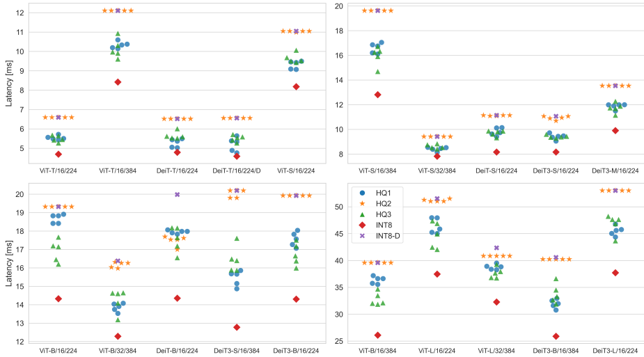
Figure 4.5: CPU-only workstation: Average Intel Xeon 5218 Gold CPU inference latency of models. Each point represents a single quantization configuration. We report the average latency of linear layers over 1000 samples.
